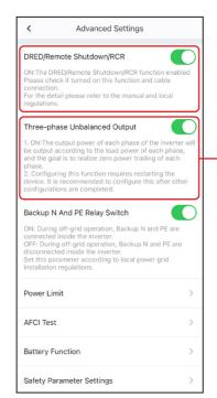
Enable **Three-phase Unbalanced Output** when the utility grid company adopts phase separate billing.
